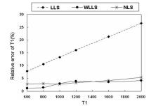
Fig. 2 Relative error of  $T_i$  using the LLS, WLLS, and NLS methods with  $SNR_0 = 100$ .
